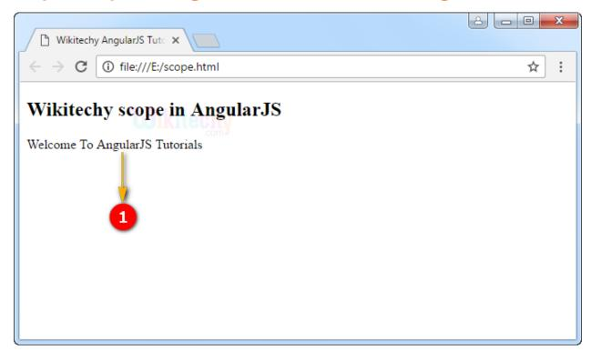
The output displays a message of a variable msg by using a ng-controller directive.
